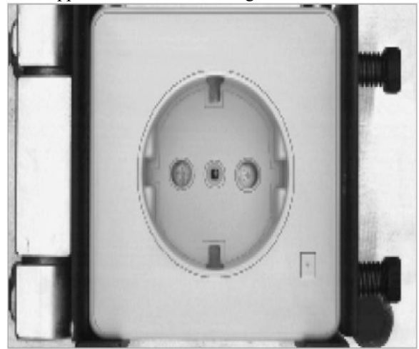
Fig.1 Digital image processing is used to verify the dimensional accuracy and examine the surface for inclusion and defects.
