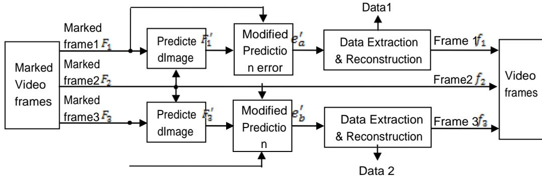
Fig. 4. Block diagram of Proposed Data extraction
